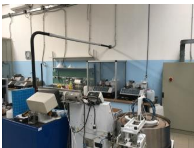
Figure 11: FILAR shop floor with lapping and polishing stations into optomechanical area
