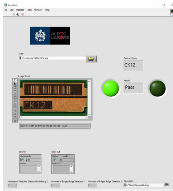
Figure 3: LabVIEW program and GUI that assess the waveguide quality of semiconductor laser devices and display the results
